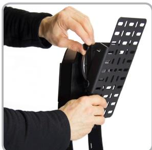
Before measurement simply slide and align lamp to center.
