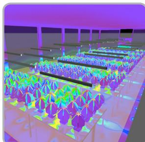
Heat map shows exact PPFD distution on any desired plane.
