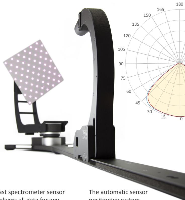
Universal bracket easily allows any lamp to be mounted.
